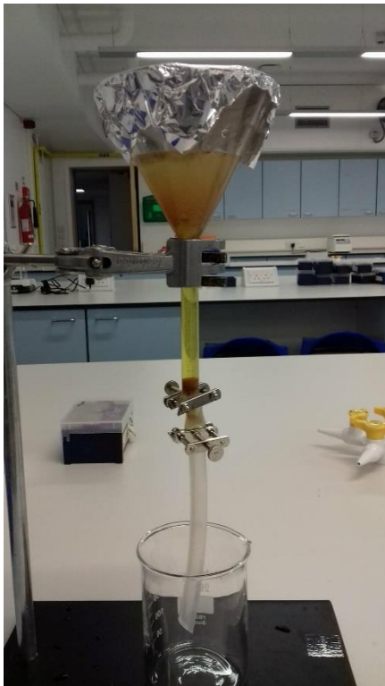
Figure 4. A density separator constructed to NOAA's guidelines.
